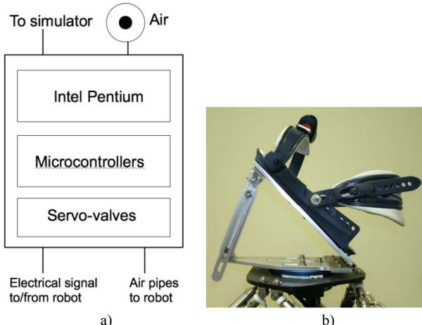
Figure 2. Hardware modifications: a) the new controller block diagram; b) ankle angle adapter. © Rutgers Tele-Rehabilitation Institute and WUSTL. Reprinted by permission.
