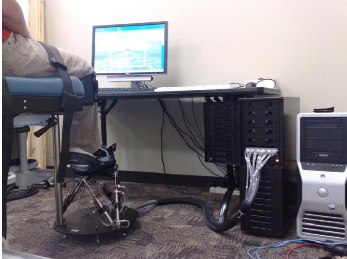
Figure 1. The Rutgers Ankle CP system installed at the clinical site. © Rutgers Tele-Rehabilitation Institute and WUSTL. Reprinted by permission.
