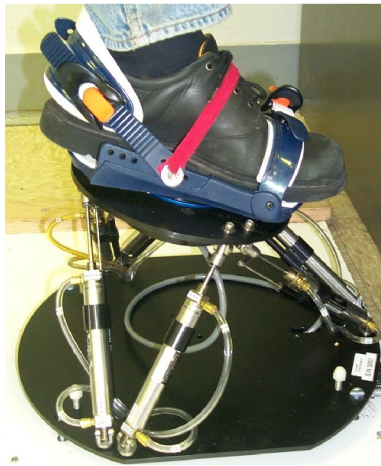
Figure 3.2: Rutgers Ankle (RA) robot [14].
