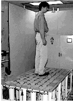
(a) Terrain Surface Simulator ALF [84]
