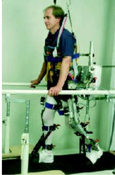
Figure 8.1: The Lokomat® gait orthosis. From the Automatic Control Laboratory, Swiss Federal Institute of Technology (ETH), Zurich, Switzerland.
