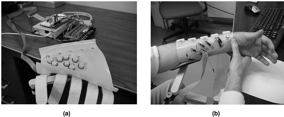
Figure 1. Sensory sleeve: a) FSR sensor with silicone foam discs line the inner surface of a sleeve. A hardware interface acquires signals from the sensor array; b) A normal subject dons the sleeve and places the arm in the tracking armrest.
