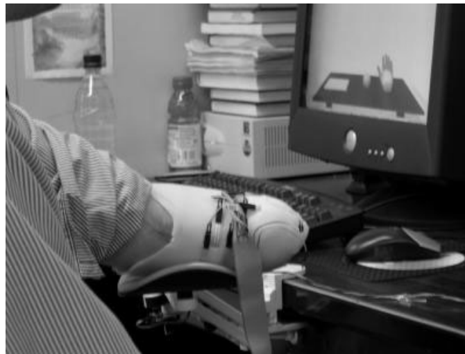
Figure 10. An amputee subject fitted with the sensing socket performing the VR experiment.
