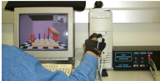
Figure 2. The VR-based orthopedic rehabilitation using a haptic glove during a peg-board exercise. © IEEE 2000.
