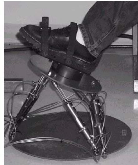
Figure 1 .The “Rutgers Ankle” Haptic Interface (Girone, et al., 1999). © ASME. Reprinted by permission.
