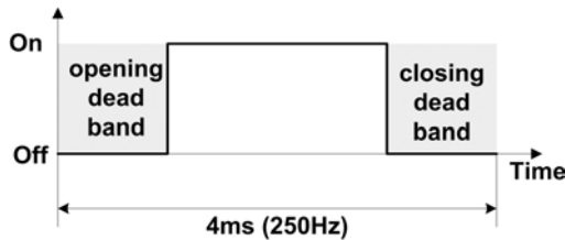
Figure 5. Dead band in a PWM Period. © Rutgers University. Reprinted by permission.
