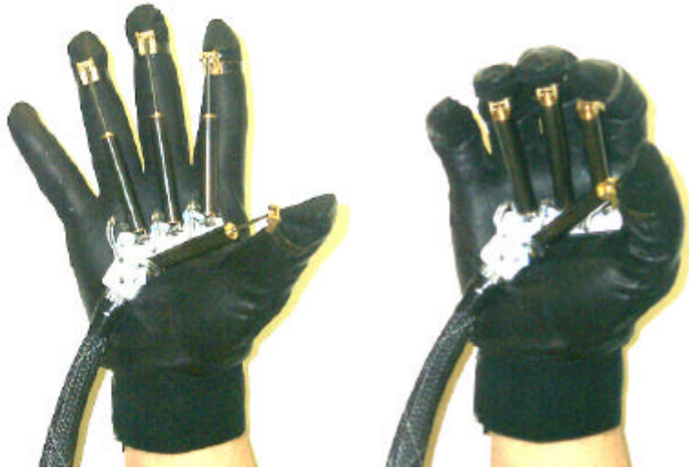
Figure 3.4: The RMII-ND master glove, a) Open hand; b) Closed hand.
