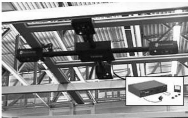
**Figure 16:** The InterSense IS-600<sup>®</sup> inertial/ultrasonic tracker. Courtesy of InterSense Co. Reprinted by permission
