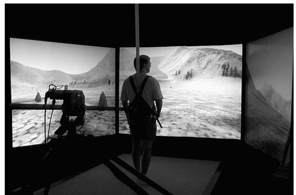
**Figure 21:** The treadport VR system. Courtesy of University of Utah CS Dept. Reprinted by permission
