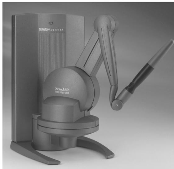
**Figure 17:** The PHANToM<sup>®</sup> desktop force feedback arm. Courtesy of SensAble Co. Reprinted by permission
