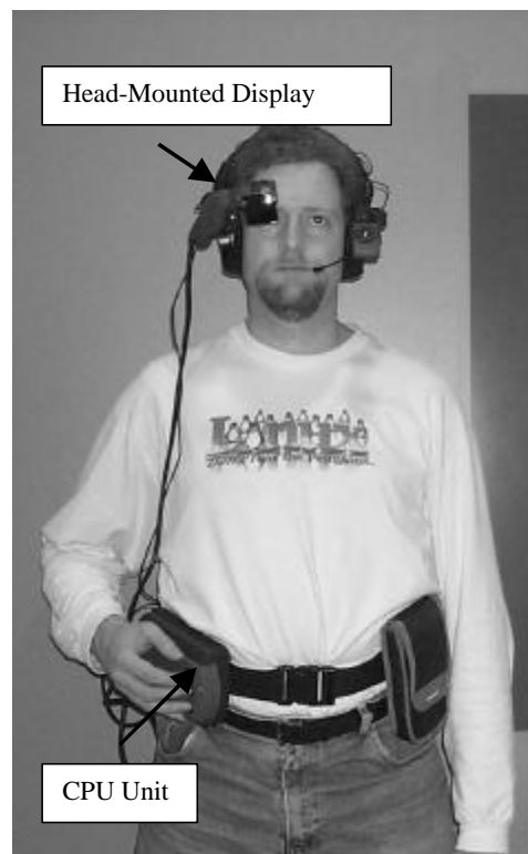
Figure 10. The Mobile Assistant IV wearable computer. Courtesy of CAIP Center. Reprinted by permission.
