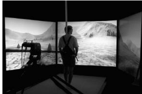
Figure 7. The treadmill with force feedback arm system developed at the University of Utah. Reprinted by permission.
