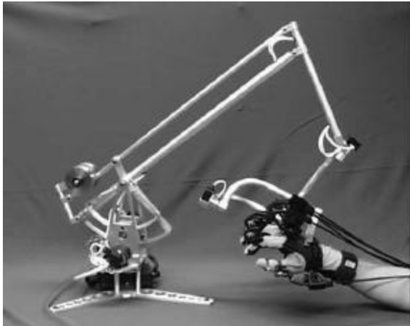
Figure 6. The CyberForce® arm coupled with the CyberGrasp glove produced by Virtual Technologies Co. Reprinted by permission.
