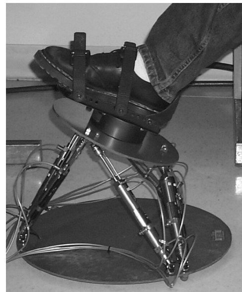
Figure 3. The "Rutgers Ankle" Haptic Interface
