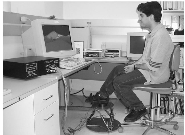
Figure 1. The "Rutgers Ankle" Orthopedic Rehabilitation System
